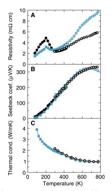
**Fig. 2.** Temperature dependence of the (**A**) resistivity, (**B**) Seebeck coefficient, and (**C**) thermal conductivity of a representative sample of  $Tl_{0.02}Pb_{0.98}Te$  and of  $Tl_{0.01}Pb_{0.99}Te$ , using the same conventions as in Fig. 1. The open and closed symbols represent data taken in two different measurement systems.
